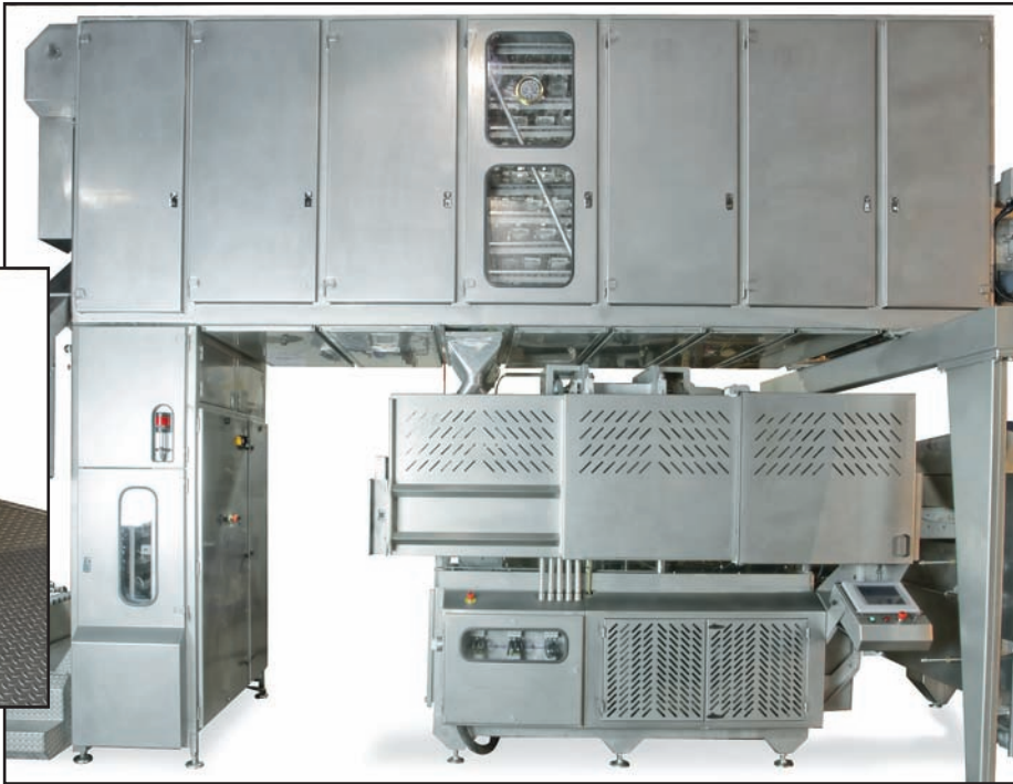
Press guard for operator protection See through windows for viewing and electrical component fault lights
