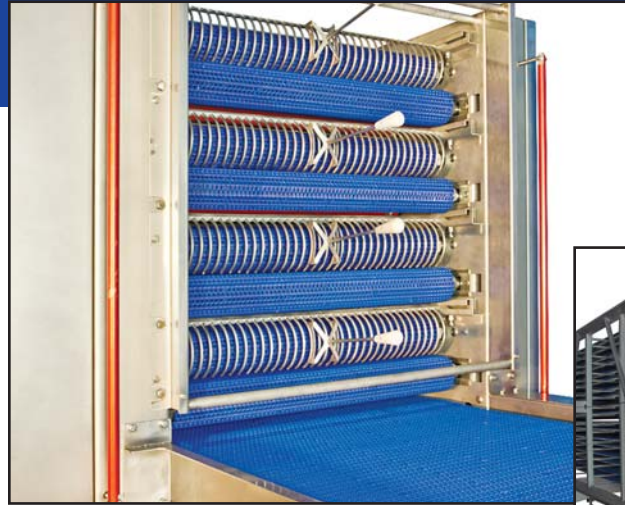
Safety Doors with external cooler chute handles for product jam clean-out
