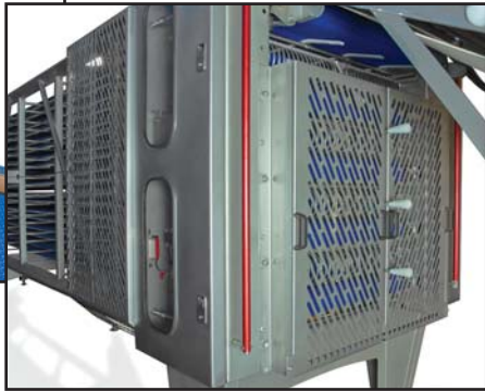
Safety Doors with external cooler chute handles for product jam clean-out
