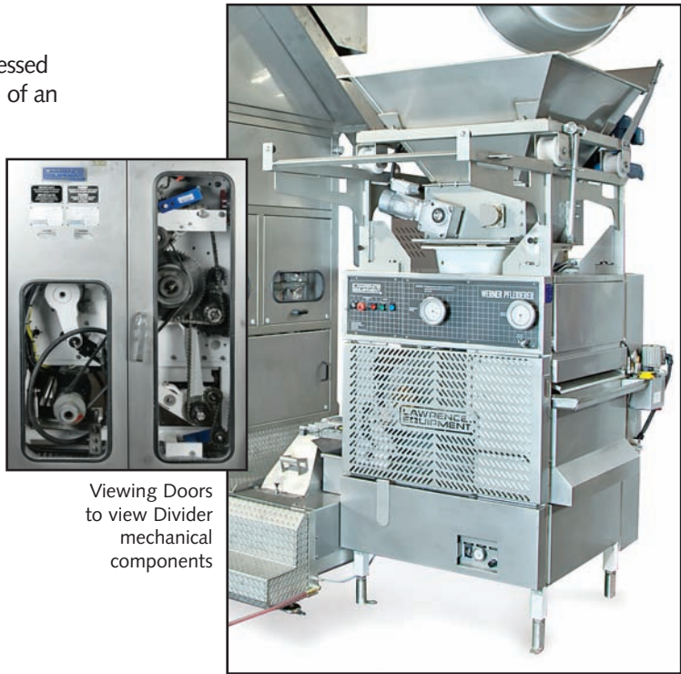
Werner and Pfleiderer TWWS with Lawrence Automatic Dough Feeder, Automatic Oiling System and Air Dryer
