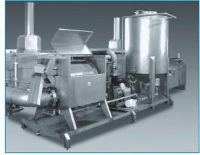
Rotary drum screen continuously removes fines from oil flow
