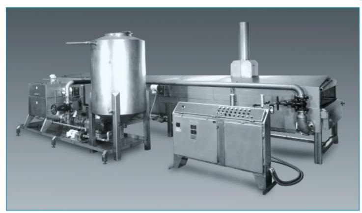
Space efficient configuration: Tank, drum screen filter & pump are built in a stainless steel oil containment pan
