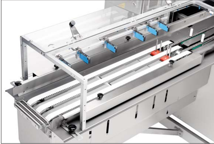
Advanced stack staging in feed reconfigures itself based on the diameters.
