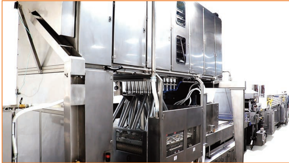
Continuous monitoring camera on critical divider to proofer transfer. Proofer exit for emergency dough ball evacuation.
