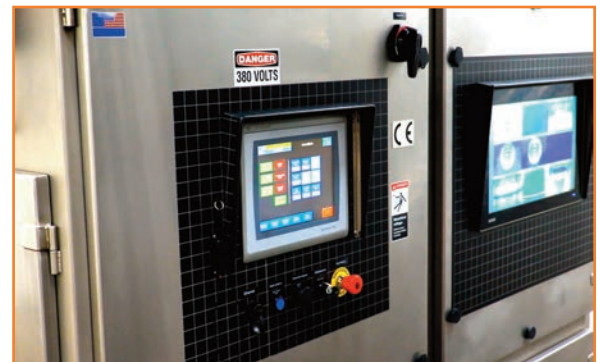
LEFT: One Touch control screen RIGHT: All camera position viewing screen
