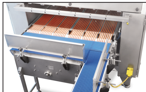
Lawrence 6-row Counter Stacker indexing into single file orientation ready for either manual bagging or automatic packaging machine interface
