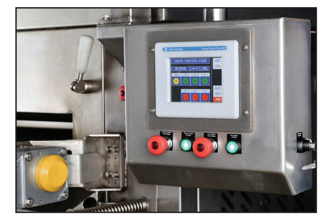
Recipe driven HMI/PLC system control
